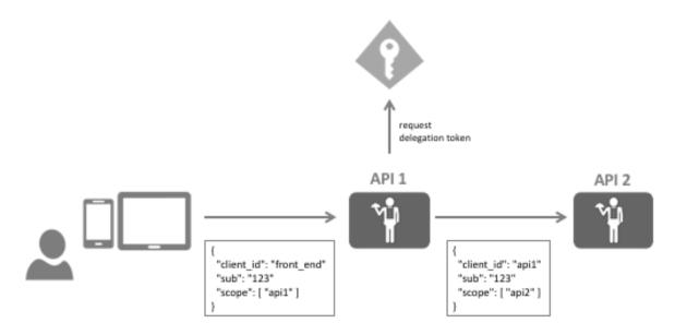
In other words, the middle tier API (API 1) needs an access token containing the user's identity, but with the scope of the back end API (API 2).
