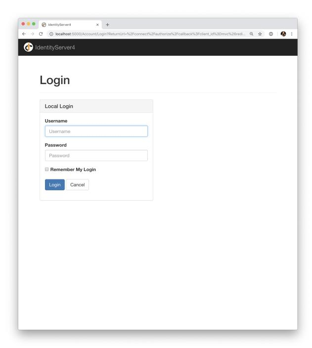
After that, the IdentityServer will redirect back to the MVC client, where the OpenID Connect authentication handler processes the response and signs-in the user locally by setting a cookie. Finally the MVC view will show the contents of the cookie.
